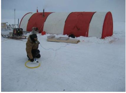
on the surface of the ice. The picture shows Alex with the receiving antenna. (The junior member of any team is always the one who goes outside.) The transmitter is under the ice a couple of metres on this side of the tent. The ice is roughly 2 m thick, and they were able to get contact at a maximum horizontal range of about 8 m. (This was just one of the experiments that they did.) They, too, were quite happy with their results.
