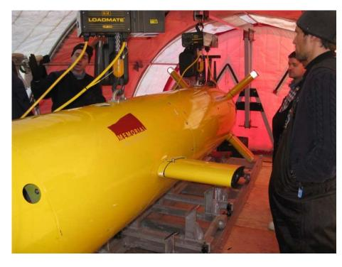
you can see the box beam holding up the electric winches. For the engineers in the crowd, the centre of the beam deflected an inch and five eighths when it took the weight. As nearly as I could tell, their only problem of the day was a battery charger that failed.
