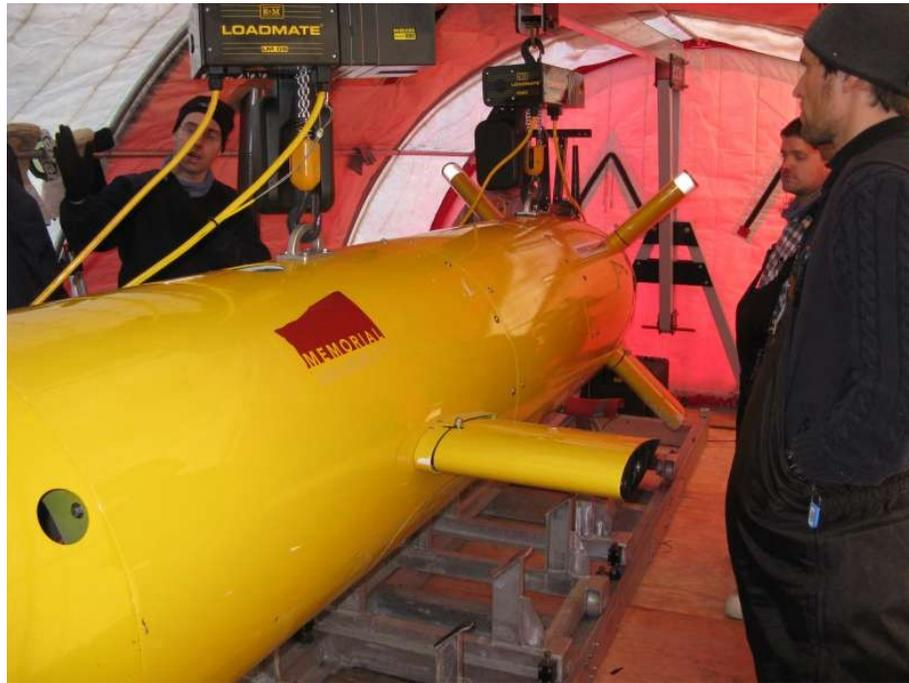
you can see the box beam holding up the electric winches. For the engineers in the crowd, the centre of the beam deflected an inch and five eighths when it took the weight. As nearly as I could tell, their only problem of the day was a battery charger that failed.
