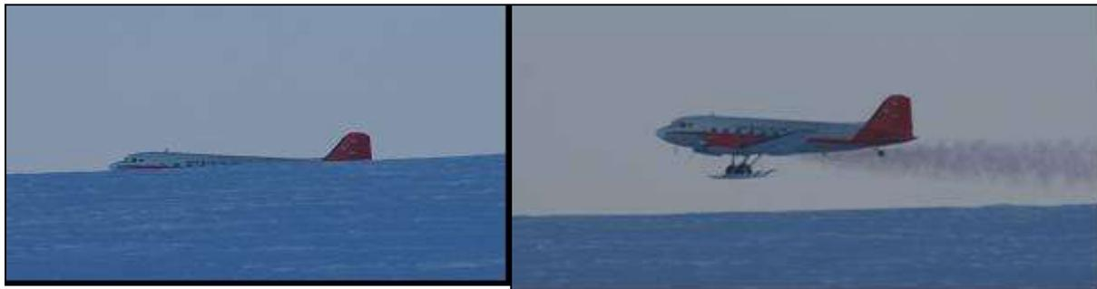
At one time we had all three aircraft circled around the fuel cache. Unloading the DC-3 is fast because it stops nose-high and the floor slopes steeply down to the rear doors.
